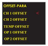
CH 1 OFFSET: TO CORRECTION TURBIDITY VALUE ON CHANNEL 1.
