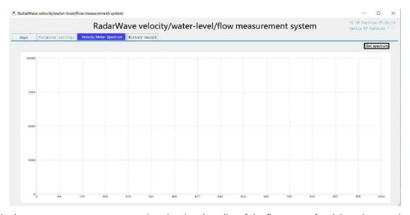
Click the button get spectrum, you can view the signal quality of the flow meter for debugging on-site.
