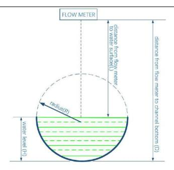
Register address to the round channel parameters
