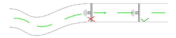
2. Avoid the sensor directly faces to the water flows with large drop
