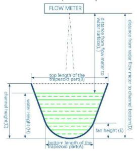
Register address to the U-shaped channel parameters
