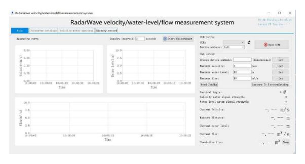
The software main window display the current water level, flow velocity, instantaneous flow, cumulative flow and other information, and it also display the reading by graph.
