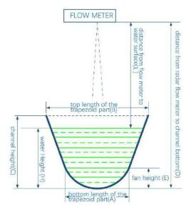
Register address to the trapezoidal channel parameters
