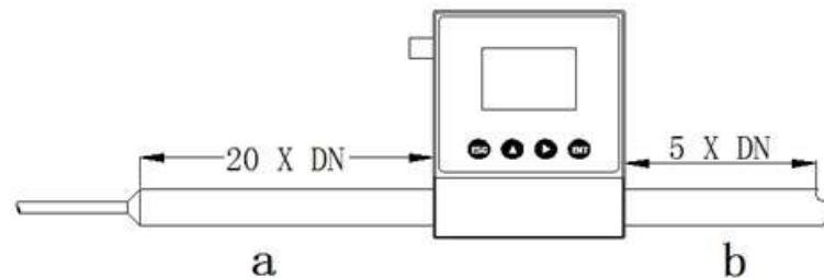
With a 90 degree joint or t-pipe:
