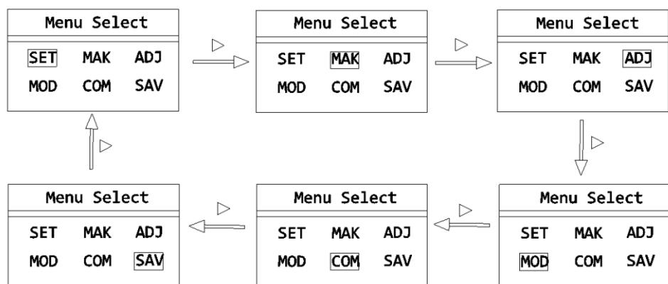
Set Basic parameters menu, remove the black rectangle to the "Settings", press "ENT" key, the password input menu appears, press "ENT" key again, a flashing cursor appears, enter the password, after the password input is completed, press "ENT" key to confirm. if the password is correct, it will directly enter into the parameter Settings menu. if the
