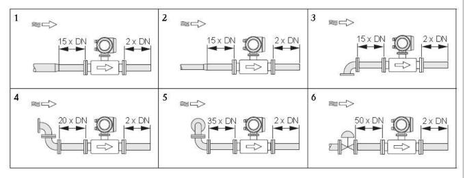
1 = Reduction, 2 = Expansion, 3 =  $90^{\circ}$  elbow or T-piece,  $4 = 2 \times 90^{\circ}$  elbow,
