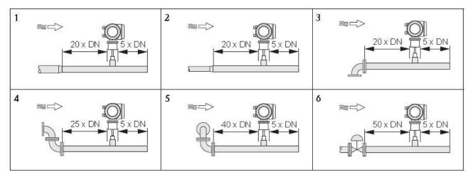
1 = Reduction, 2 = Expansion, 3 =  $90^{\circ}$  elbow or T-piece, 4 =  $2 \times 90^{\circ}$  elbow,
